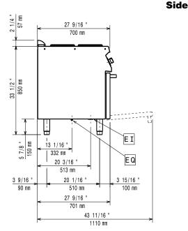
EI = Electrical inlet (power) **EQ** = Equipotential screw
